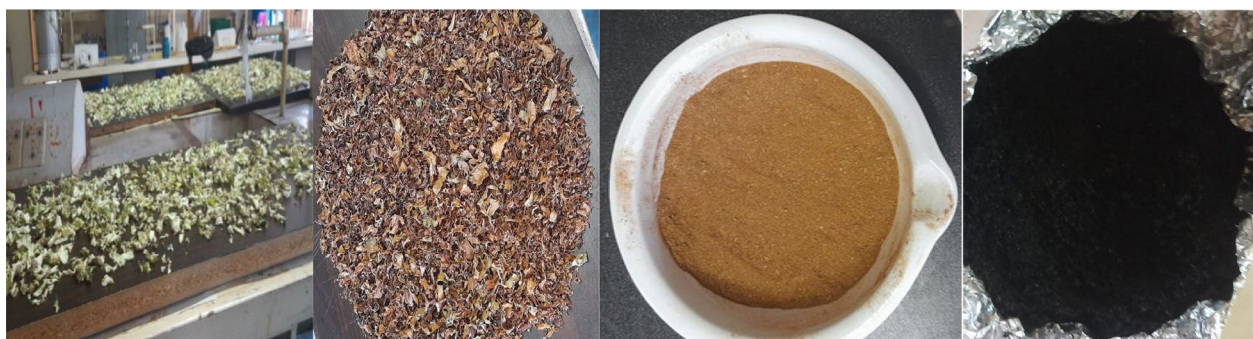
Fig. 1 Preparation of activated carbon derived from cabbage waste
