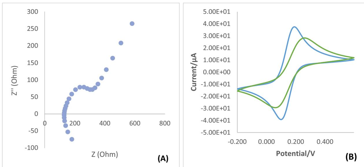
**Fig. 8** **A** Graphene electrode (G1) response spectra after EIS application on the bare electrode. **B** Overlaying of the CV scans for both graphene electrode (blue) and carbon electrode (green). Graphene electrode (G1) response scan after CV application on the bare electrode corresponds to the scan in blue color, whereas Cyclic voltammetry (CV) after SPCE pretreatment (bare electrode measurements) is in green color (Fig. 2A)
