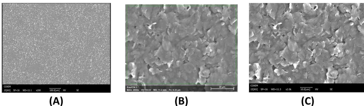
**Fig. 5** **A** Scanning Electron Microscope image of bare screen-printed carbon electrode (working electrode) surface. **B** Scanning Electron Microscope image of CMA-modified screen-printed carbon electrode (working electrode) surface. **C** Scanning Electron Microscope image of screen-printed carbon electrode surface, after incubation of the working electrode with the ciprofloxacin aptamer
