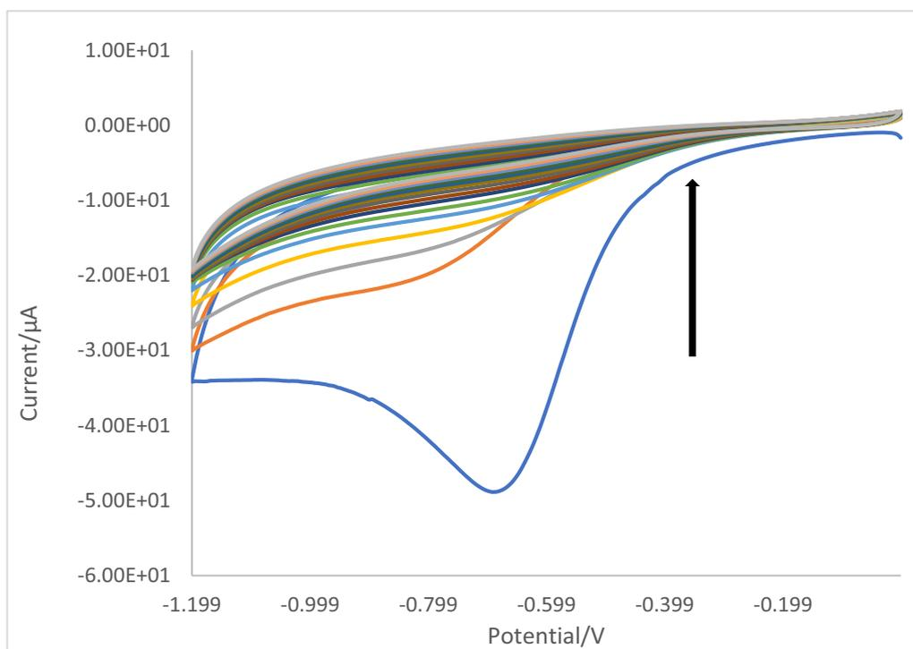
**Fig. 3** Scans using cyclic voltammetry (CV) for CMA deposition. This CV scan shows 15 CV cycles, used to deposit diazonium salt on the surface of screen-printed carbon electrodes
