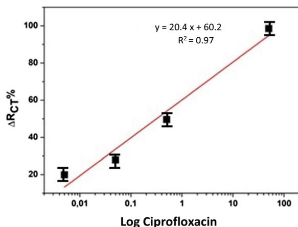
**Fig. 7** Calibration curve representing the EIS response of aptasensor, after incubation in different concentrations of ciprofloxacin
