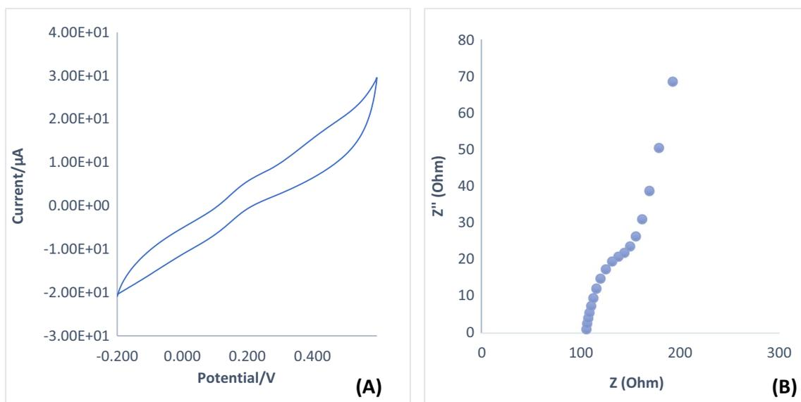
**Fig. 10** **A** Graphene electrode (G1) response scan after CV application, following CMA deposition. **B** Graphene electrode (G1) response spectra after EIS application, following incubation with the aptamer
