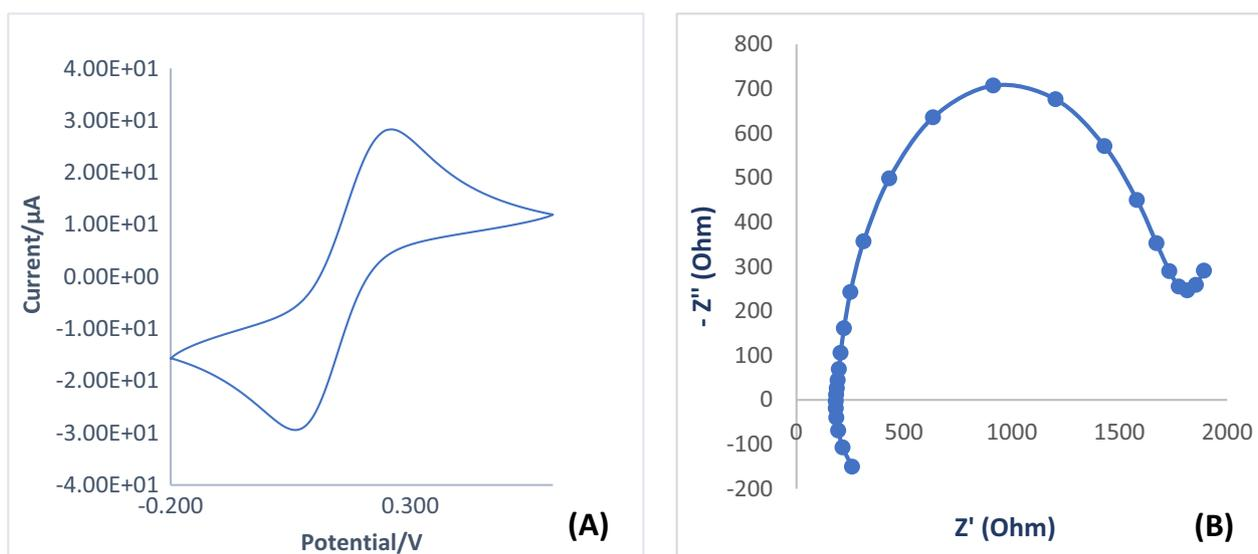
**Fig. 2** **A** Cyclic voltammetry (CV) after SPCE pretreatment (bare electrode measurements) The oxidation peak's potential value for this CV scan is  $0.259 \text{ V} \pm 0.005$ . **B** Electrochemical Impedance Spectroscopy (EIS) spectra after SPCE pretreatment (bare electrode measurements).
