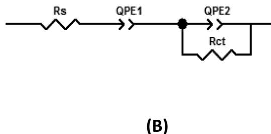
**Fig. 6** **A** Nyquist plot showing the EIS response of aptasensor after incubation in different concentrations of ciprofloxacin. **B** Equivalent circuit used for the mathematical fitting of the EIS responses of the aptasensor
