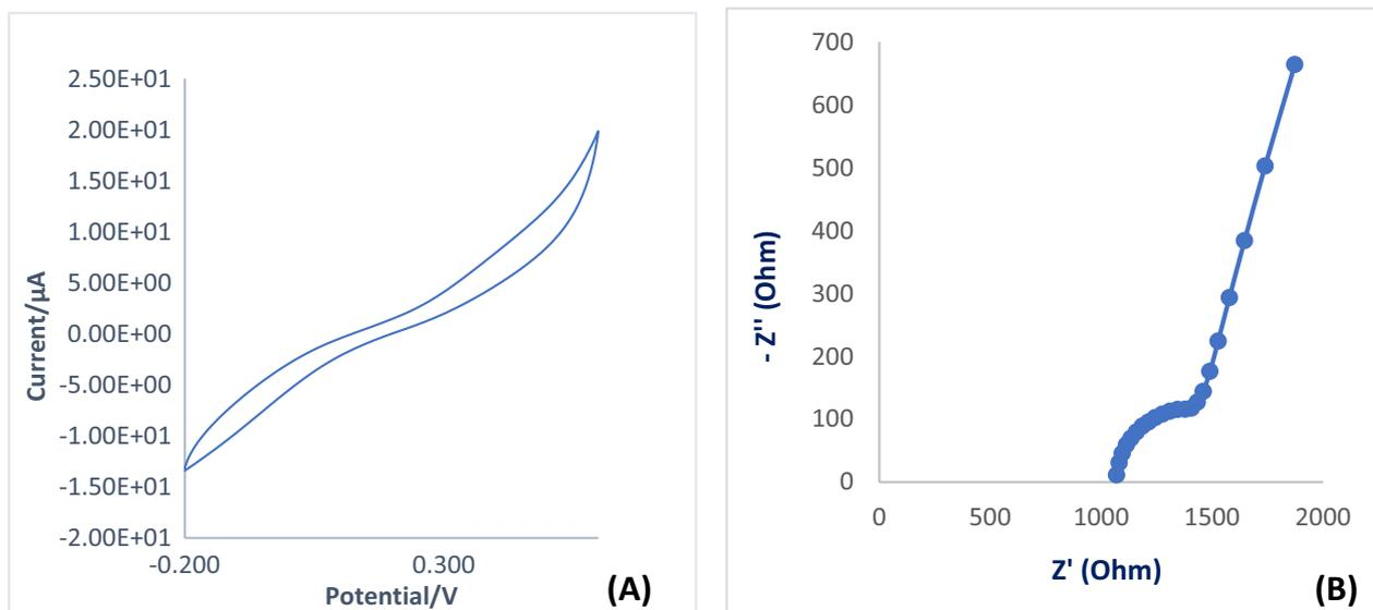
**Fig. 4 A** Cyclic Voltammetry (CV) scan after CMA deposition. This figure represents a CV scan, following the previous diazonium salt deposition. **B** Electrochemical Impedance Spectroscopy (EIS) spectrum after aptamer incubation. This figure represents an EIS spectrum, following the incubation of the CMA-modified electrode with the ciprofloxacin aptamer
