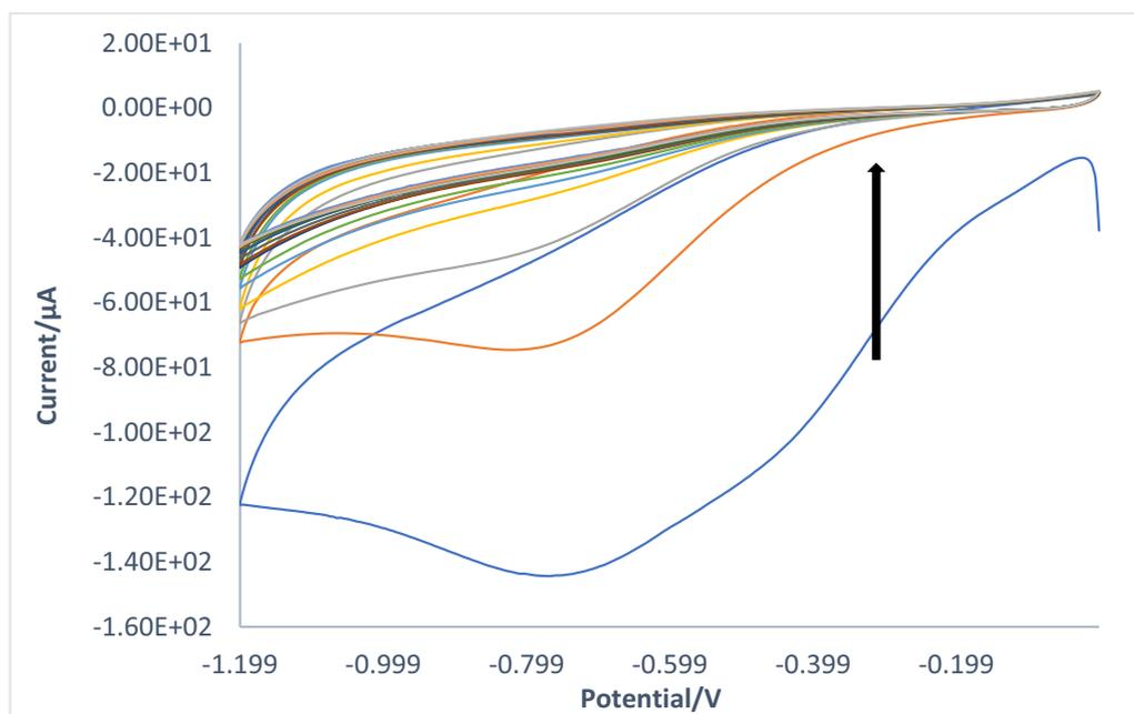
**Fig. 9** Graphene electrode (G1) cyclic voltammetry (CV) scan for CMA deposition. This scan shows 15 CV cycles, used to deposit diazonium salt on the surface of graphene electrodes
