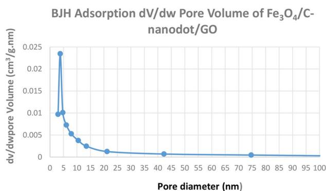
**Fig. 8** BJH pore size distribution of  $\text{GO}/\text{Fe}_3\text{O}_4/\text{C-nanodot}$
