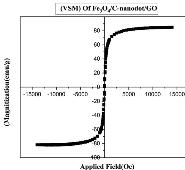
**Fig. 5** Vibrating sample magnetometer (VSM) Of Fe<sub>3</sub>O<sub>4</sub>/C-nanodot/GO
