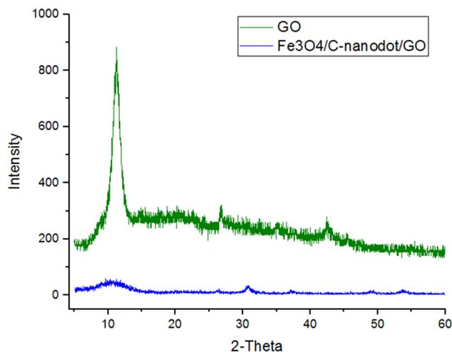
**Fig. 4** XRD spectra of GO, Fe<sub>3</sub>O<sub>4</sub>/C-nanodot/GO
