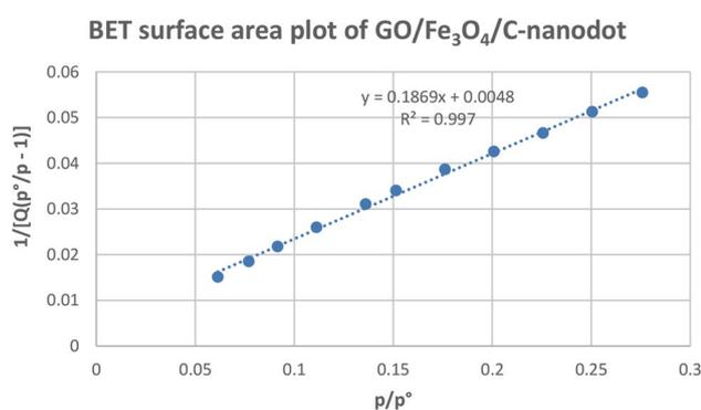
**Fig. 7** BET surface area plot of  $\text{GO}/\text{Fe}_3\text{O}_4/\text{C-nanodot}$
