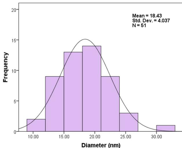
**Fig. 3** The average particle size of GO/PANI adsorbent was obtained using ImageJ software
