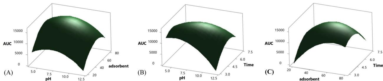
**Fig. 9** Surface plot of absorption of methamphetamine (a) pH vs. adsorbent and (b) adsorbent vs. time (c) pH vs. time for GO/PANI composite
