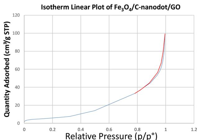
**Fig. 6** A BET N2 adsorption/desorption isotherms of  $\text{Fe}_3\text{O}_4/\text{C-nanodot}/\text{GO}$
