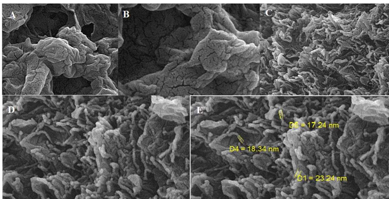
**Fig. 2** Scanning electron microscopy (SEM) of: (A) GO at  $500\text{ nm}$  scale, (B) GO at  $200\text{ nm}$  scale, (C) GO-polyaniline composite at  $500\text{ nm}$  scale, (D) GO-polyaniline composite at  $200\text{ nm}$  scale, (E) GO-polyaniline composite at  $200\text{ nm}$  scale by indicating density
