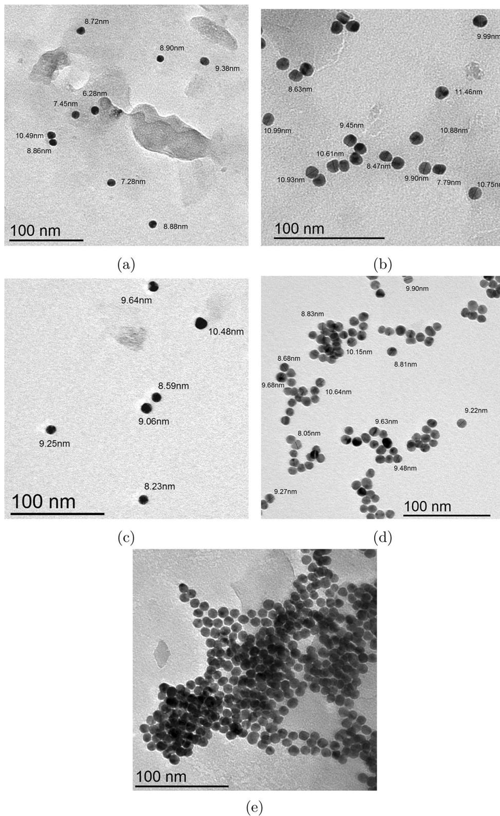
**Fig. 1** High resolution transmission electron microscope (HRTEM) images of gold nanospheres, alone (a), with tobramycin nano-concentration (b), with alendronate micro-concentration (c), with memantine micro-concentration (d), with tobramycin micro-concentration (e)
