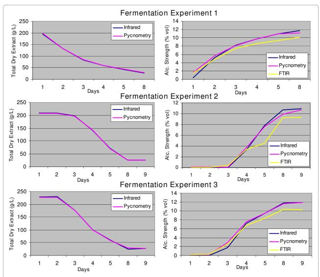
Figure 3 Three wine fermentations were followed using the portable infrared spectrometer in comparison to reference analysis using distillation and pycnometry. The alcoholic strength was also determined using a laboratory FTIR analyzer.
