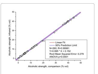
**Figure 2** Linear correlation between comparison results and infrared spectroscopic results for the determination of alcoholic strength in 260 different alcoholic beverages (beer, wine, and spirits).
